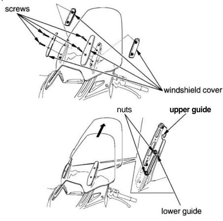
1. Remove the windshield cover by removing the screws.
