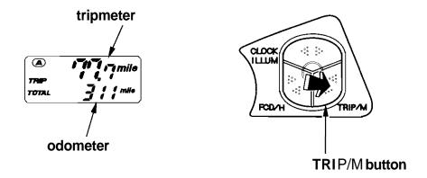
The tripmeter will show mileage in two sub modes, "tripmeter A" and "tripmeter B."
