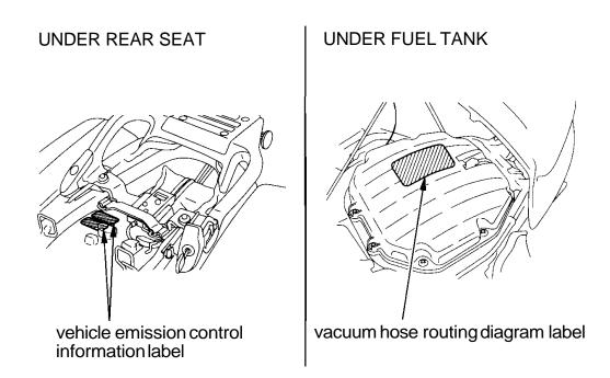
The Vehicle Emission Control Information label is attached on the rear fender under the rear seat.
