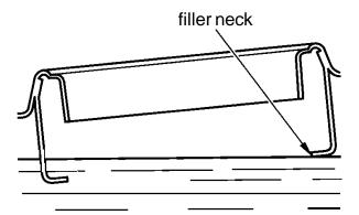
**3.** Add fuel until the level reaches the bottom of the filler neck. Avoid overfilling the tank. There should be no fuel in the filler neck.
