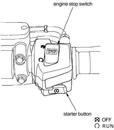
The engine stop switch is used to stop the engine in an emergency. To operate, push the switch to the OFF position. The switch must be in the RUN position to start the engine, and it should normally remain in the RUN position even when the engine is OFF.
