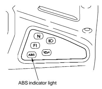
If the ABS indicator light blinks while riding, stop the motorcycle in a safe place and turn off the engine. Turn the ignition ON again. The light should come on, and then go off after you ride the motorcycle at speeds above 6 mph  $(10\,k\,m/h)$  If it does not go off or if it blinks again, ABS is not functioning. However, the Linked Braking System will still provide normal stopping ability. However, you should have the system checked by your Honda dealer as soon as possible.
