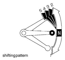
Your motorcycle has five forward gears in a one-down, four-up shift pattern which is coordinated with a hydraulically actuated clutch system.
