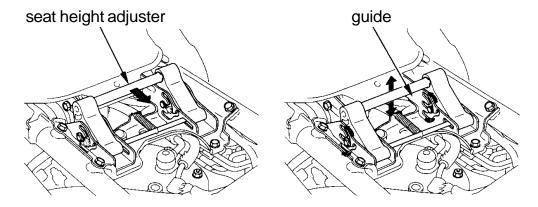
Be sure to align the hole in the rear of the front seat with the adjuster when install the front seat.
