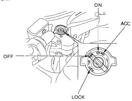
The ignition switch is used for starting and stopping the engine (page 53) and to lock the steering for theft prevention (page 63). Insert the key and turn it to the right for the ON and ACC (accessory) positions. Push down on the key and turn it to the left to the LOCK (steering lock) position.
