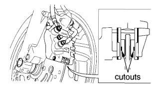
Always inspect both pads in both the right and left front brake calipers. Check the cutouts in each pad. If either pad is worn to the cutout, replace both pads as a set. See your Honda dealer for this service.
