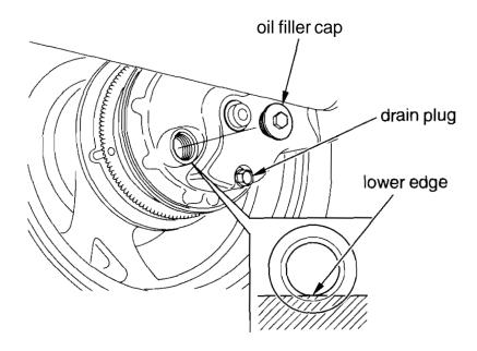
Change the oil with the final drive at normal operating temperature to assure complete and rapid draining.
