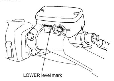
Check that the fluid level is above the LOWER level mark. If the fluid level is below the LOWER level mark, it indicates fluid leakage. See your Honda dealer for repair.
